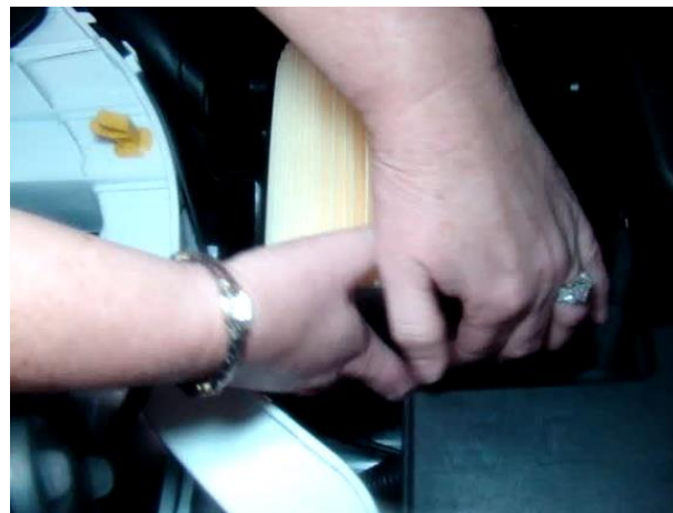
Figure 6: Seat closed end of Filter in housing
